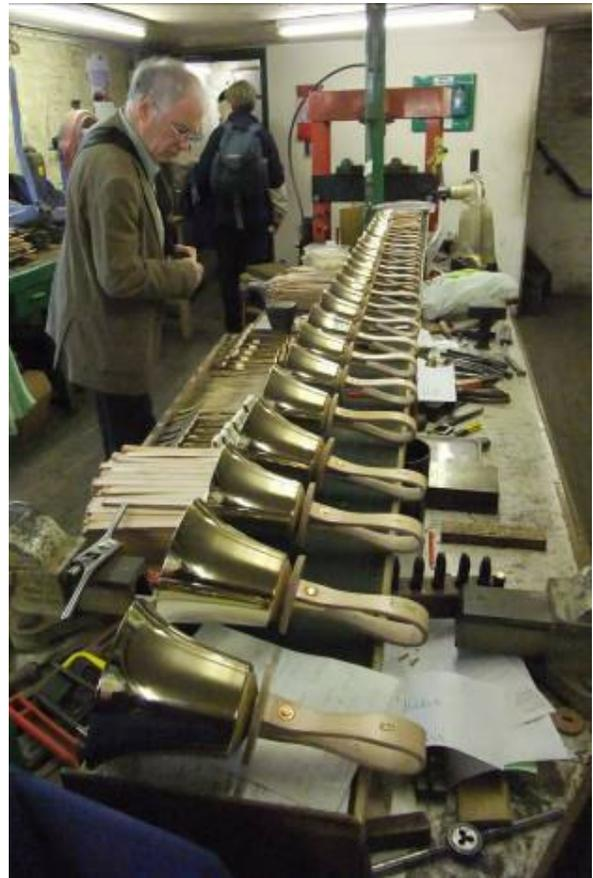
We then came down a level to the Handbell department which concentrated on tuning and buffing of the bells, the manufacture of the handles out of leather and the assembly of the clappers. On entrance to this small but long room we noticed a long line of 40 finished
